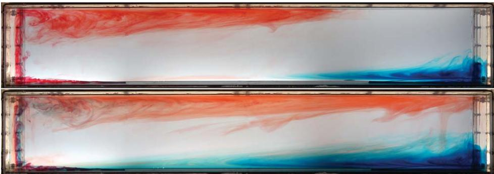
FIGURE 4. Flow visualization of circulation in regime 3.  $R_Q = -0.14$ , left plume dominant. The dye was injected as described for figure 3. Time elapsed between the two frames was approximately 13 min.
