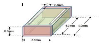
engaged in the development of silicon solar cells, one of the solar cells to be used in sixjunction tandem stack. Key challenges to develop the silicon cells are the small dimensions of  $2.5 \times 8 mm^2$  and the need to transfer light with energy of less than 1.1ev to the cells stacked underneath it.
