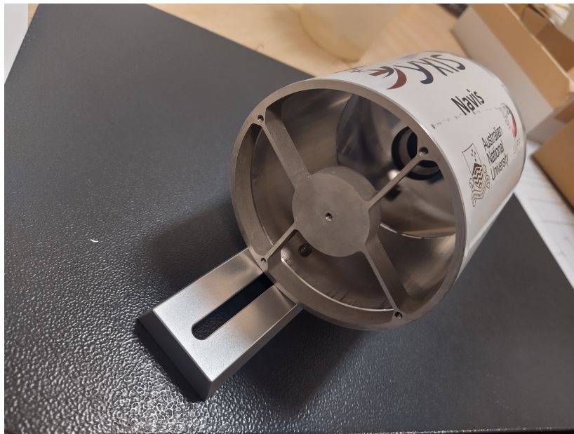
Figure 5.6: A photograph of one of the diamond-turned aluminium telescopes.
