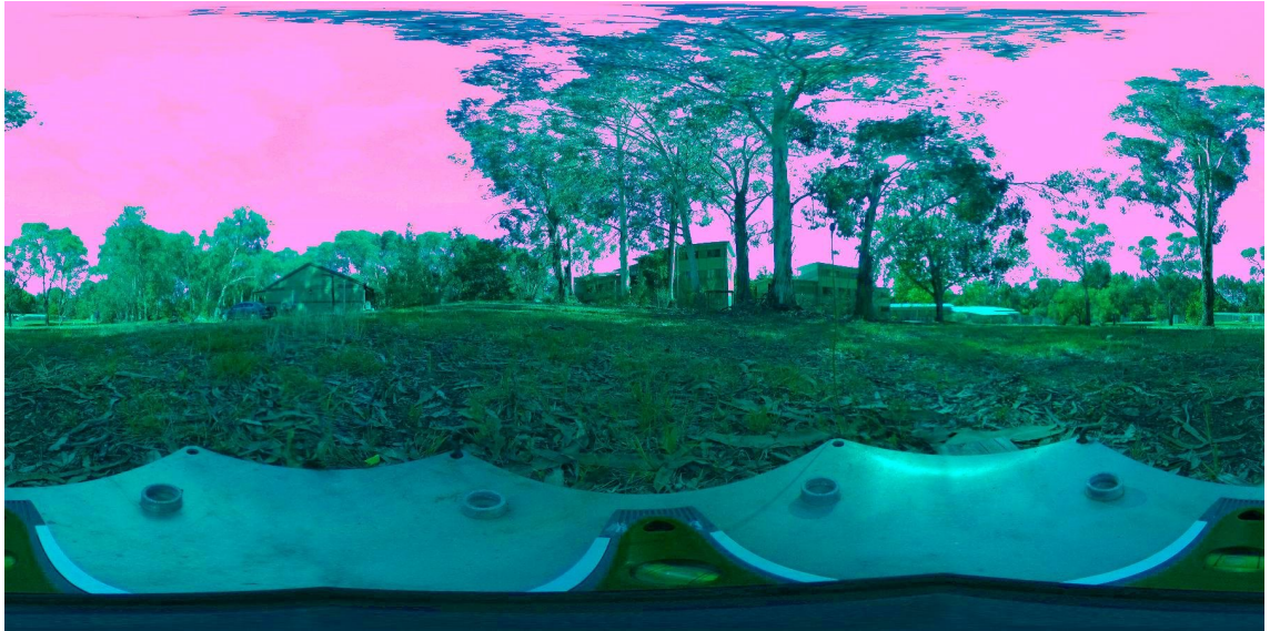
Fig. 42: Familiar location, red component and sky features removed, UV added above the skyline. The magenta sky is due to the otherwise unused red channel being utilised to represent the UV illumination.
