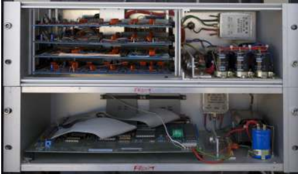
Figure 2. Part of the electronics station at a siderostat. The upper module is the FSM consisting of four hand-wired circuit boards and a power supply. The module beneath it is the single-board computer and its power supply.
