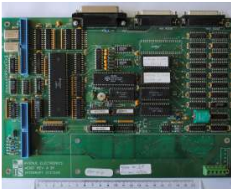
Figure 1. One of the single-board computers used as embedded processors in SUSI.
