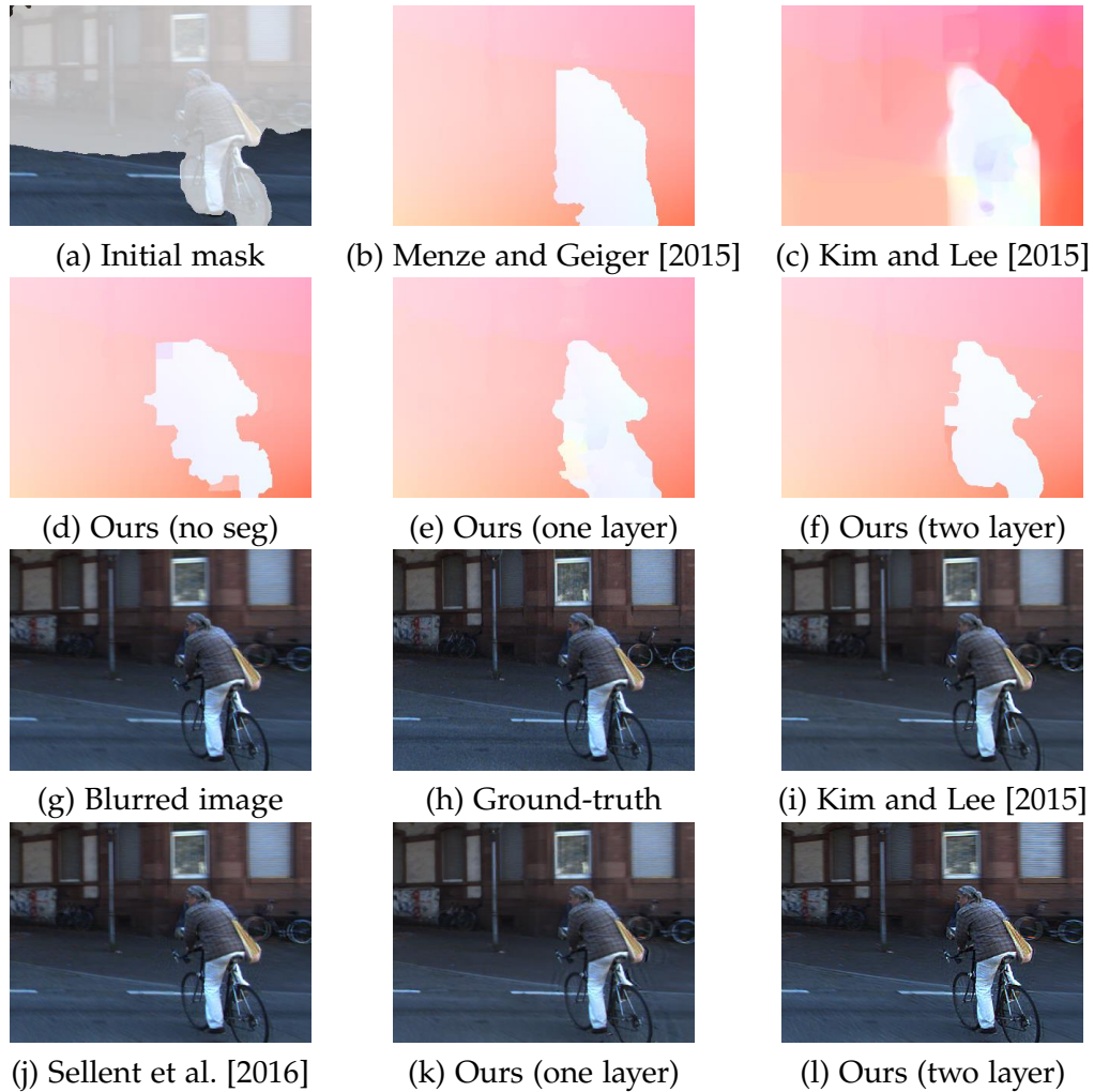
Figure 4.4: Scene flow results for an outdoor scenario. (a) and (g) The initial segmentation and blurred reference image from BlurData-1 . (b) Estimated flow by Menze and Geiger [2015]. (c) Estimated flow by Kim and Lee [2015]. (d)-(f) Our flow estimation result. (d) Without semantic segmentation. (e) With semantic segmentation, one layer StereoSLIC. (f) With semantic segmentation, two-layer StereoSLIC. (h) The ground-truth latent image. (i) Deblurred result by Kim and Lee [2015]. (j) Deblurred result by Sellent et al. [2016]. (k) and (l) Our deblurred result. (k) Without semantic segmentation. (l) With semantic segmentation. The results show that our two-layer StereoSLIC could preserve edge information. Compared with both these state-of-the-art methods, our method achieves competitive performance. Best viewed in colour on the screen.
