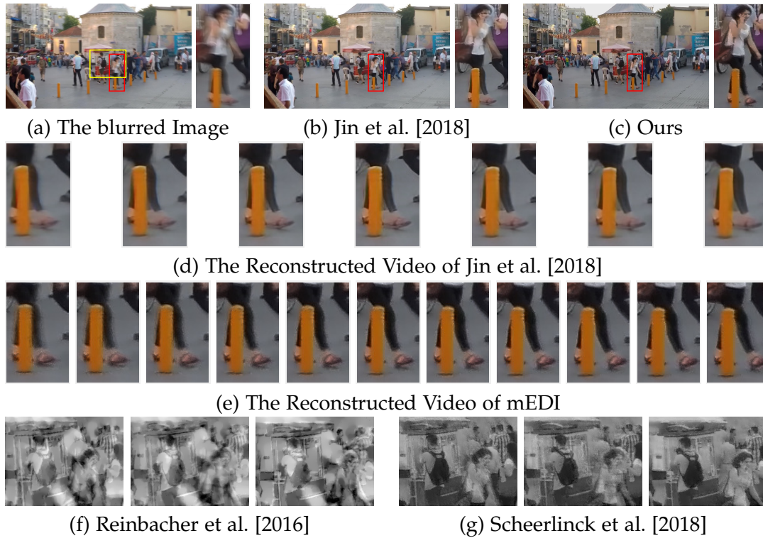
Figure 6.7: An example of the reconstructed result on our synthetic event dataset based on the GoPro dataset Nah et al. [2017]. Nah et al. [2017] provides videos to generate blurred images and event data. (a) The blurred image. The red close-up frame is for (b)-(e), the yellow close-up frame is for (f)-(g). (b) The deblurring result of Jin et al. [2018]. (c) Our deblurring result. (d) The crop of their reconstructed images and the frame number is fixed at 7. Jin et al. [2018] uses the GoPro dataset added with 20 scenes as training data and their model is supervised by 7 consecutive sharp frames. (e) The crop of our reconstructed images. (f) The crop of Reinbacher et al. [2016] reconstructed images from only events. (g) The crop of Scheerlinck et al. [2018] reconstructed image, they use both events and the intensity image. For (e)-(g), the shown frames are the chosen examples, where the length of the reconstructed video is based on the number of events. (Best viewed on screen).
