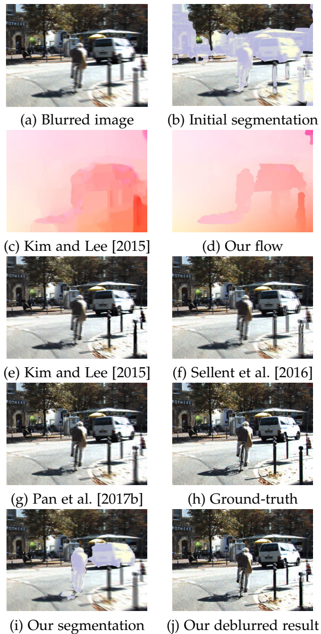
Figure 4.1: Stereo deblurring, scene flow estimation and moving object segmentation results with (a) and (b) as input. (a) Blurred image. (b) Initial segmentation prior. (c) Flow estimation by Kim and Lee [2015]. (d) Our flow estimation result. (e) Deblurring results by Kim and Lee [2015]. (f) Stereo deblurring results by Sellent et al. [2016] which uses Vogel et al. [2015] to estimate scene flow. (g) Deblurring results by Pan et al. [2017b]. (h) Ground-truth latent image. (i) Our moving object segmentation result. (j) Our stereo deblurring result. Best viewed in colour on the screen.
