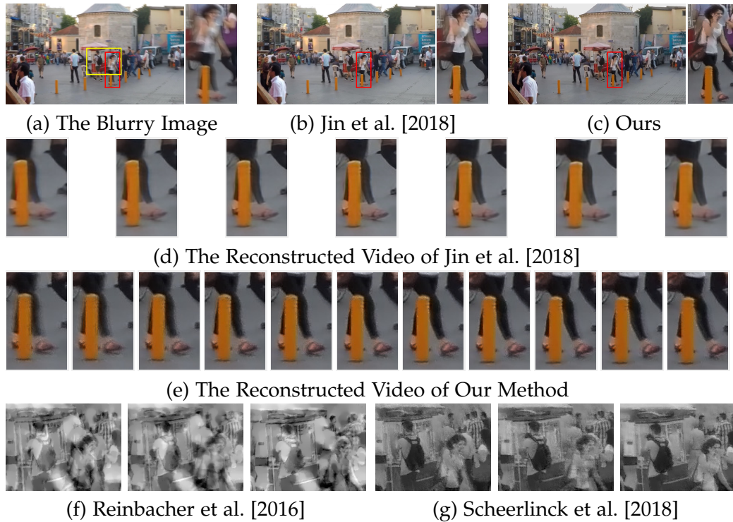
Figure 5.7: An example of the reconstructed result on our synthetic event dataset based on the GoPro dataset Nah et al. [2017]. Nah et al. [2017] provides videos to generate the blurry images and event data. (a) The blurry image. The red close-up frame is for (b)-(e), the yellow close-up frame is for (f)-(g). (b) The deblurring result of Jin et al. [2018]. (c) Our deblurring result. (d) The crop of their reconstructed images and the frame number is fixed at 7. Jin et al. [2018] uses the GoPro dataset added with 20 scenes as training data and their model is supervised by 7 consecutive sharp frames. (e) The crop of our reconstructed images. (f) The crop of Reinbacher Reinbacher et al. [2016] reconstructed images from only events. (g) The crop of Scheerlinck Scheerlinck et al. [2018] reconstructed image, they use both events and the intensity image. For (e)-(g), the shown frames are the chosen examples, where the length of the reconstructed video is based on the number of events.
