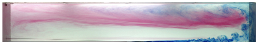
Figure 1. Enhanced full-depth convective circulation (side view looking horizontally through the flow) at t \approx 6 min after a sudden increase in heat input. Blue dye injected for t > 0 displaces red dye injected for t < 0 . Cooling and heating are applied over the left- and right-hand halves of the base, respectively. The initial thermally-equilibrated circulation is visualized in figure 2a.
