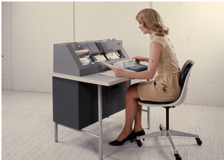
An IBM 029 Card punch. (Unfortunately, not an ANU one.) Photo courtesy of IBM, ©International Business Machines Corporation.
