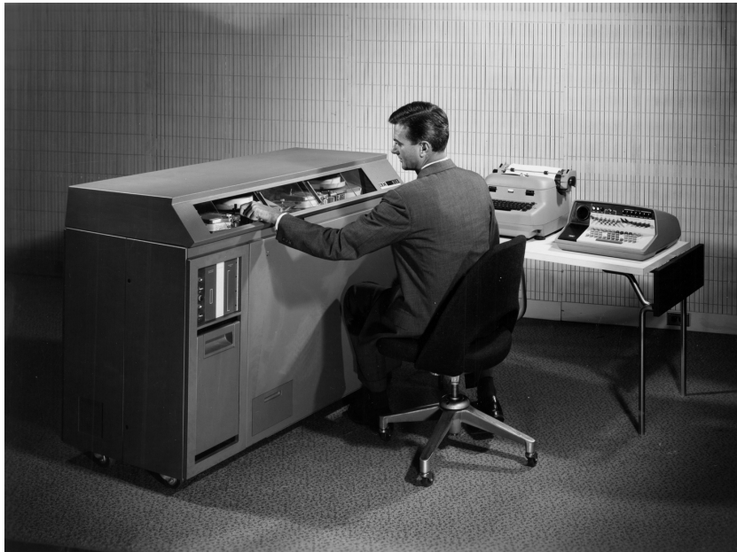
An IBM 610, of the same type as ANU's first computer. Programs were represented on paper tape rather than in memory (i.e. it was not a stored-program computer.) The door at the lower left of the cabinet conceals the fold-out plugboard. Photo courtesy of IBM, ©International Business Machines Corporation.
