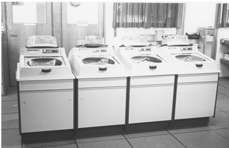
1975: Resembling a laundrette, a row of removable disk drives for the Univac 1100/42. Photo from A Pictorial History of the CSC.
