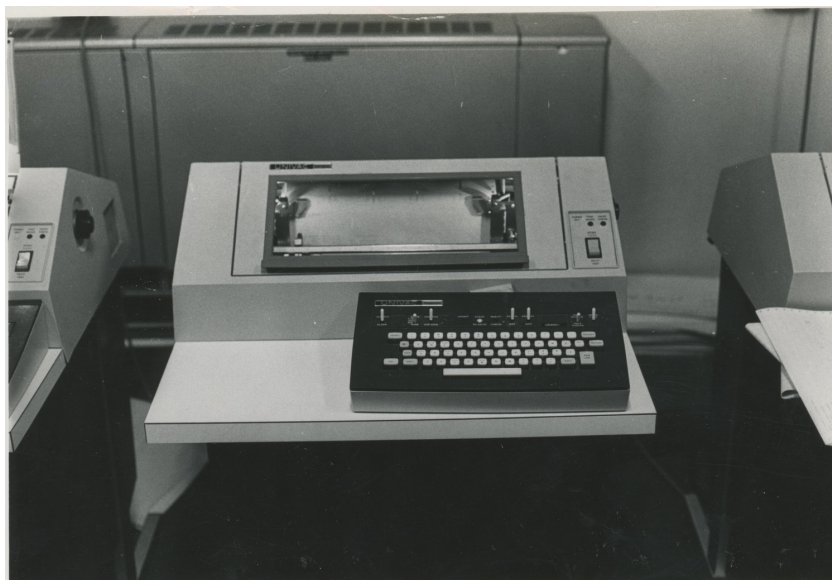
A Univac DCT 500 printing terminal, part of a cluster in G Block, across the road from the Menzies Library. Photo: David Hawking
