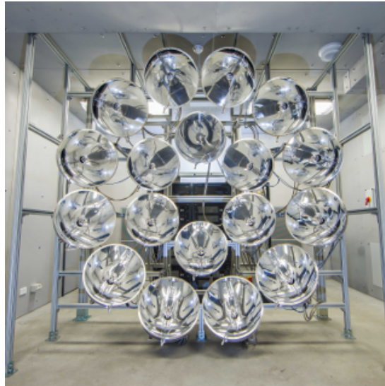
Figure 2.3: Photograph of the multi-source high-flux solar simulator (HFSS) at the Australian National University (ANU) [66].
