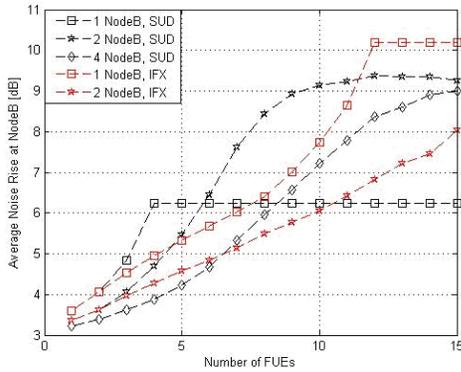
Fig. 2. Noise rise at uplink enterprise femtocells
