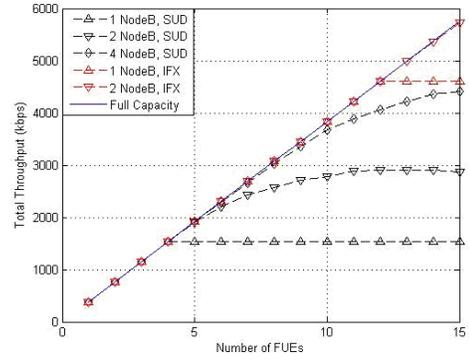
Fig. 1. Uplink capacity for enterprise femtocells
