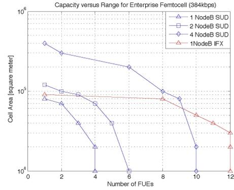
Fig. 3. Uplink capacity vs. coverage for enterprise femtocells
