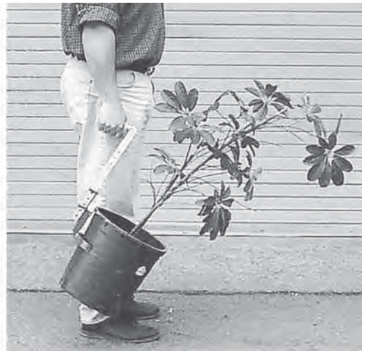
Figure 36-2. (A) Picking up and carrying large potted plants in this manner increases the risk of low back and upper-extremity injuries. (B) This device, used as an ergonomic intervention for nursery workers, reduces the need to bend in order to pick up potted plants; it also has a handle designed to decrease stress on the upper extremities. (Courtesy of University of California Davis.)
