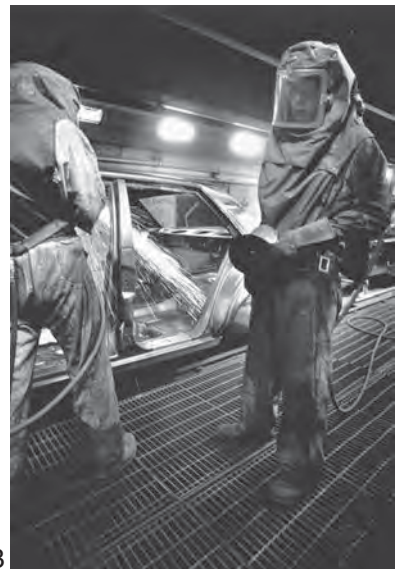
Figure 19-2. Current work practice rules require significant personal and environmental protection in situations of lead exposure: (A) Lead battery worker is protected mainly by local exhaust ventilation. (B) Automobile lead grinder is protected by air-supplied hood and floor exhaust ventilation. (Photographs by Earl Dotter.)
