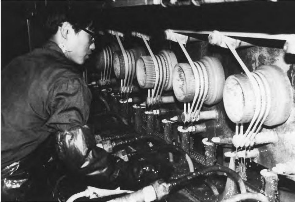
Figure 23-2. A worker tends machines that spool rayon thread from carbon disulfide. Worker exposure to carbon disulfide was high until this process was enclosed, which reduced worker exposure and, by recycling the carbon disulfide, saved the company a substantial amount of money. (Photograph by Barry S. Levy.)
