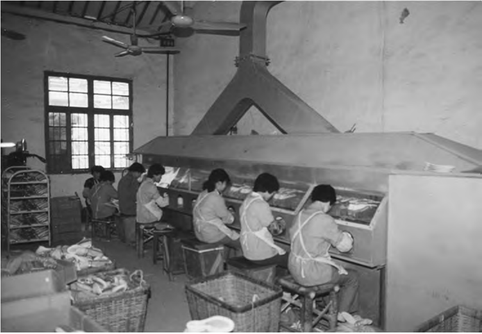
Figure 26-6. A glovebox enclosure system prevents solvent exposure to workers gluing shoes. (Photograph by Barry S. Levy.)
