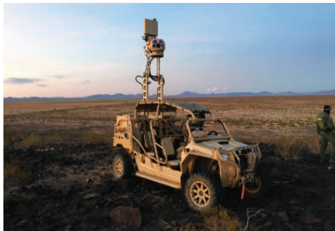
FIGURE 2. This light tactical reconnaissance and surveillance vehicle by FLIR, the LTV-X, carries a complementary sensor array that can include NIR, SWIR, thermal, laser rangefinding, and radar devices. (Courtesy of FLIR)
