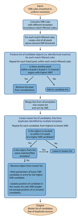
Figure 10. Flowchart describing the detailed procedure of our line search algorithm utilizing MF3D. The input is an S/N cube, and the output is a list of line features characterized by a feature S/N, which accounts for the total S/N evaluated through the template that gives the highest value.
