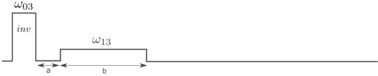
Figure 5.2: Temporal pulse sequence used for the direct gain measurement. The ensemble was initialized in the ground state |0\rangle , using the ensemble preparation method outlined in §4.3. The amplitude profile of the inversion pulse inv was shaped by convolving a top-hat function with a Gaussian function. The inversion pulse was centered at frequency \omega_{03} (see Figure 3.6), and chirped with a 300 kHz bandwidth for 8 \mu\text{s} duration. A delay time of a=3.5 \mu\text{s} was included before the probe, which was applied at \omega_{13} for duration of b=10 \mu\text{s} . To construct the gain profile the probe was stepped in \pm 50 kHz increments around \omega_{13} .
