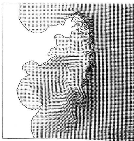
Figure 1: This computer model of flow past Bass Point (35°S), a 4-km wide headland near Sydney, shows attached eddies and a vortex street in the headland wake (adapted from [4]).
