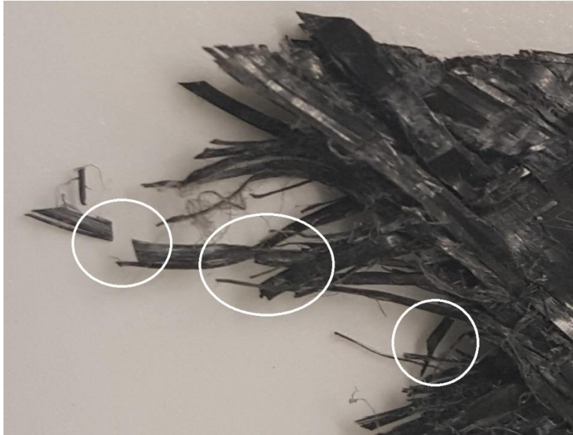
Figure 5.24 Pull-outs and fracture of tapes and fibrils in a 1.0 mm \pm 45^\circ SRPP tensile test specimen after failure. Examples of fractured tapes and fibrils are highlighted. Direction of load is horizontal in the image.
