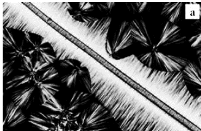
Figure 2.9 Polarised optical microscopy of the fibre-matrix interface of an SRPP formed by introducing fibre into a molten matrix at 167°C [121, Fig. 2a].
