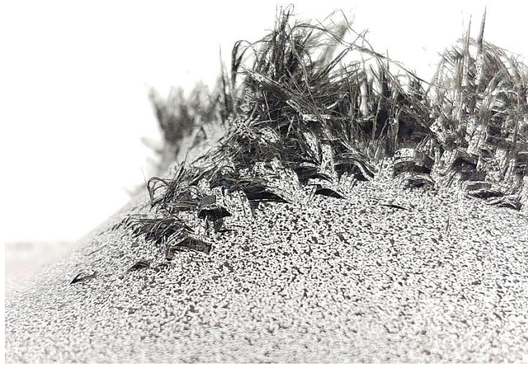
Figure 6.8 Side-view of the outer surface of a specimen, showing fibril pull-outs.
