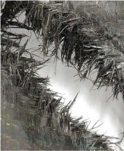
Figure 6.5 Fibril pull-outs along a diagonal failure path from the centre of a specimen.
