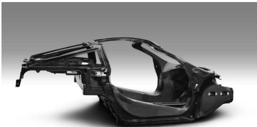
Figure 1.2 Carbon fibre-reinforced composite component in the body of McLaren 720S. [8]
