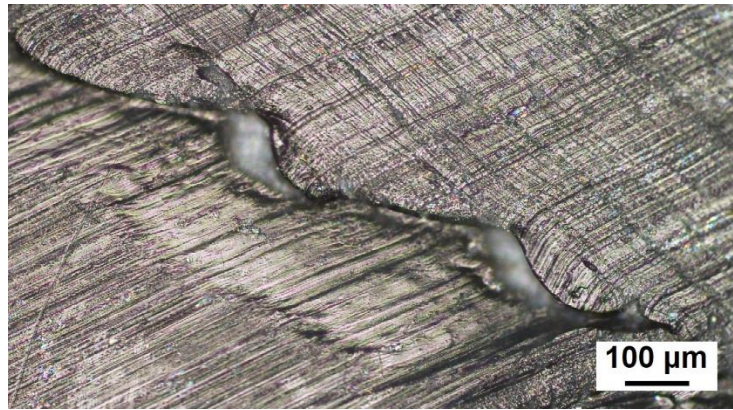
Figure 5.12 Optical micrographs of boundary cracks in 0.3 mm \pm 45^\circ SRPP tensile test specimens.
