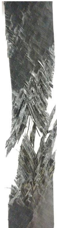
Figure 5.9 Separation of a 0.6 mm 30^\circ/60^\circ specimen after failure.
