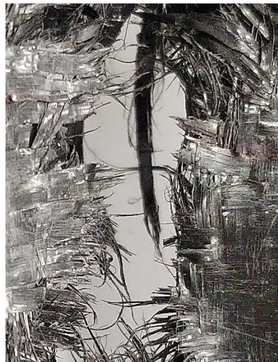
Figure 6.3 Close up of failure at the centre of the specimen shown in Figure 6.2e.
