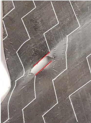
Figure 5.36 Failures along a boundary between 30° and 60°-tapes in a 0.3 mm 30°/60° SRPP tensile test specimen. White lines indicate boundaries between 30° and 60°-tapes and red lines on either side of the damage represent the same tape boundary.
