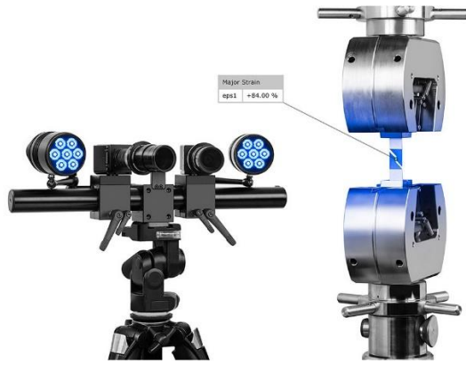
Figure 3.13 ARAMIS, a commercial digital image correlation system provided by GOM GmbH [218].
