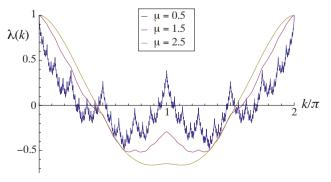
**Figure 4.** The structure function (24) of the Weierstrass random walk step probability density function (23). In each case, b = 2, and we choose a values so that so that  $\mu = \ln(a)/\ln(b)$  takes the values 0.5 [blue (most irregular) curve], 1.5 (red curve) and 2.5 (gold curve)
