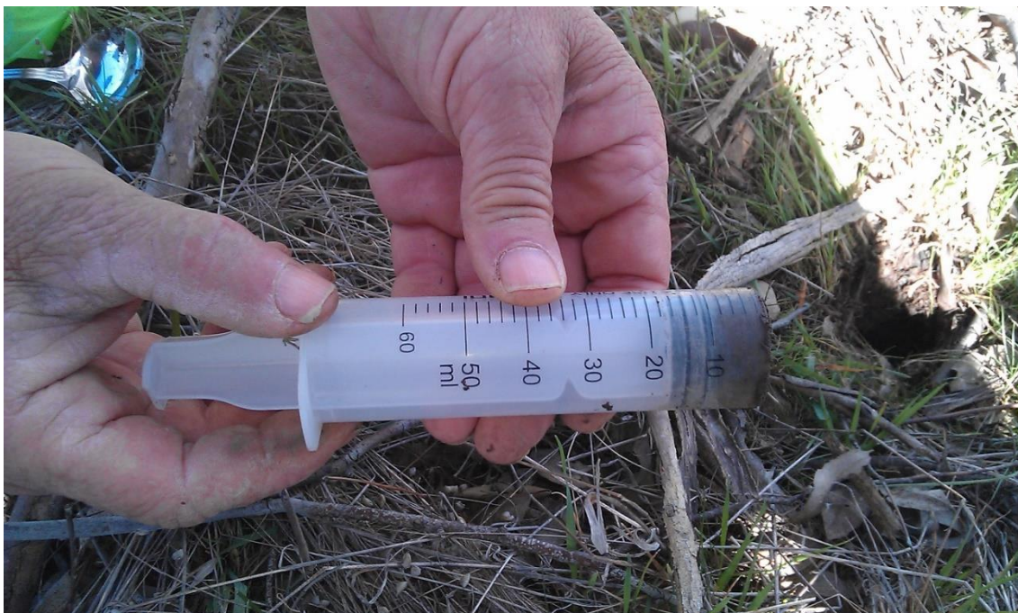
Figure S2. Method used to collect ‘under-pit’ samples – a 50mL syringe with the end cut off is pushed into the soil at the base of the pit up to the 10mL mark, giving a sample of approximately 10mL.
