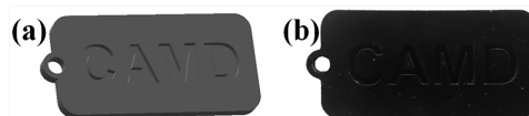
Figure 7. (a) 3D model of keyring and (b) 3D printed keyring (64.0 mm × 30.0 mm × 3.6 mm) using 15-DAAQ/TEAOH/R-Br (0.5%/2%/2%, wt %) as a photoinitiating system for the polymerization of the 3D resin.
