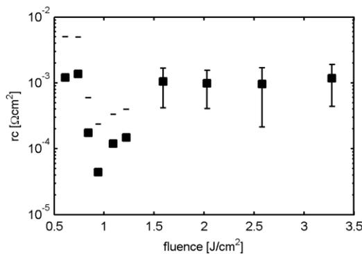
**Figure 7:** Contact resistance derived from TLM measurements of Excimer doped areas.
