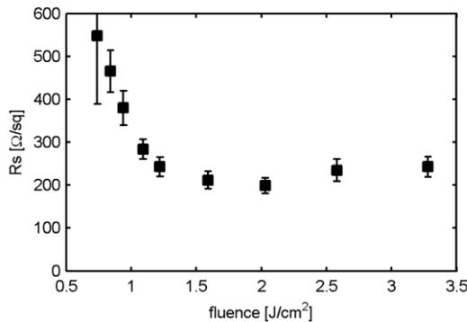
**Figure 6:** Sheet resistance derived from TLM measurements of Excimer doped areas.
