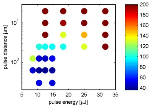
**Figure 3:** Sheet resistance [ $\Omega/\square$ ] of 532 nm DPSS laser doped areas from a  $\text{Al}_2\text{O}_3/\text{TiO}_2$  stack layer.
