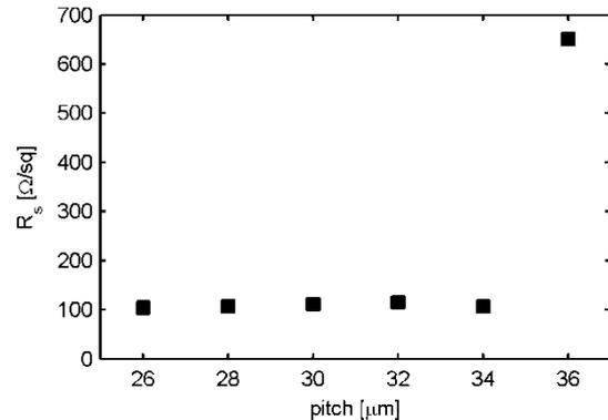
**Figure 5:** Sheet resistance of  $2.1 \text{ J}/\text{cm}^2$  excimer laser doped boxes from single  $\text{Al}_2\text{O}_3$  layer with varying pulse pitch
