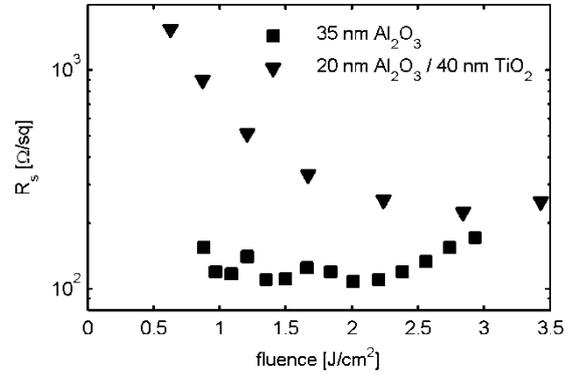
**Figure 4:** Sheet resistance for (quasi) single excimer laser pulses
