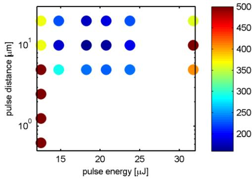
**Figure 2:** Sheet resistance [ $\Omega/\square$ ] of 532 nm DPSS laser doped areas from a single  $\text{Al}_2\text{O}_3$  layer.
