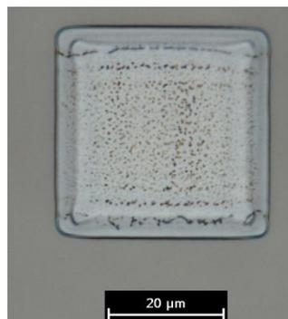
**Figure 1:** Microscope image of an Excimer laser doped square with a fluence of  $\sim 1.6$   $\text{J}/\text{cm}^2$
