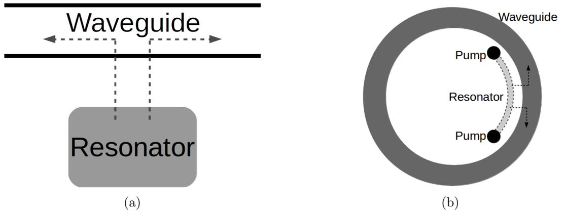
Figure 3.14: Schematics of a resonator side-coupled to a waveguide. (a) resonator side-coupled to a waveguide, (b) schematic illustrating how a pair of pump spots form a sector WGM resonator which is side-coupled to WGMs. We may consider the WGMs as waveguide modes because the centripetal potential confines them near the mesa boundary.
