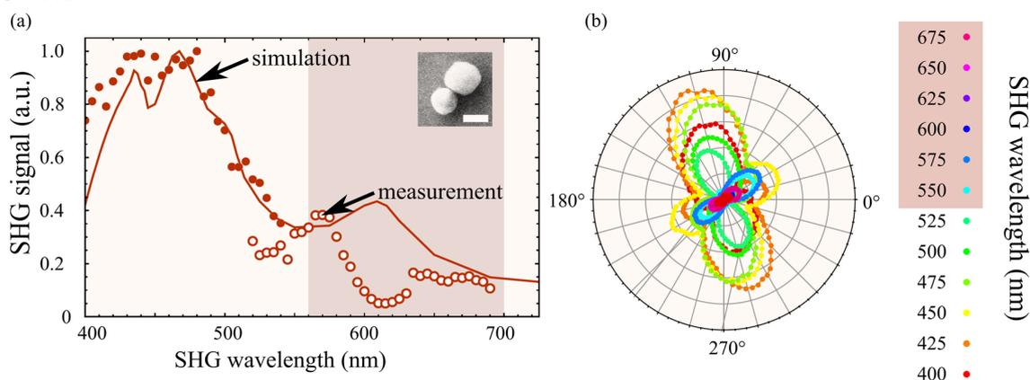
Fig. 2. (a) Normalized SHG signal of the nanodimer (inset) as a function of the second-harmonic wavelength. The solid red line shows the modeled spectrum and the red dots are the measurements points (filled laser, empty OPO range). SEM micrograph of the nanodimer in the inset, scale bar 200 nm. (b) Measured polar dependence of the normalized SHG signal from the same nanodimer. Reshaping range is highlighted in red.
