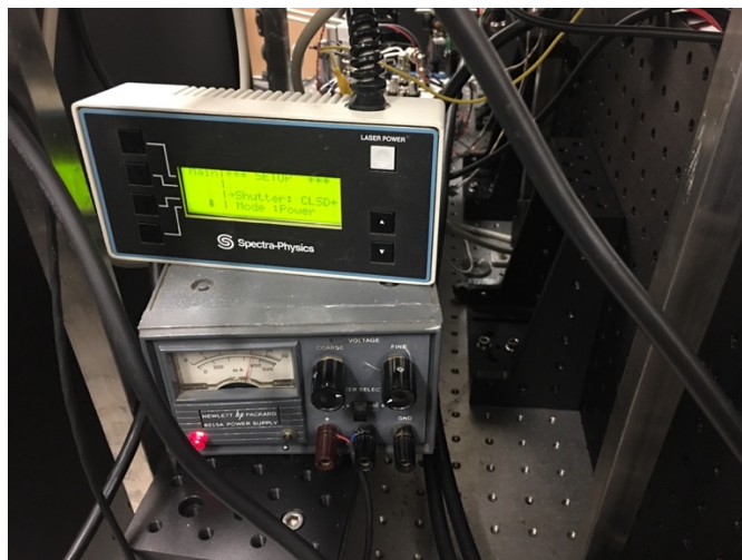
Fig. A.1 Laser controller above and the mechanical shutter control below.
