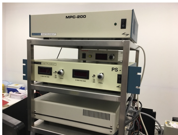
Fig. A.2 Devices above the bench, from top to bottom are the stage controller, GaAsP detector power supply, PMT power supply and mode lock controller.
