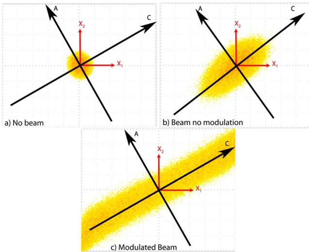
Fig. 2. Display of the oscilloscope used for measuring the noise and correlation. The  $x$  and  $y$  axis display the photocurrent generated by detectors 1 and 2, respectively. Any correlated noise will appear on the diagonal axis labeled C; any uncorrelated noise will appear equally on the A and C axes. (a) The laser is turned off, (b) the laser beam at 8 mW without modulation, and (c) the laser beam at 8 mW and maximum modulation.
