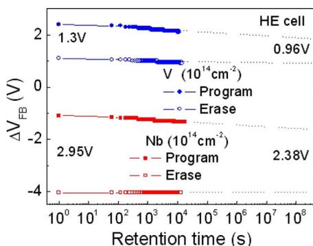
FIG. 4. (Color online) Retention characteristics of HE memory cells containing V and Nb ions of  $10^{14}$   $\text{cm}^{-2}$  fluence.
