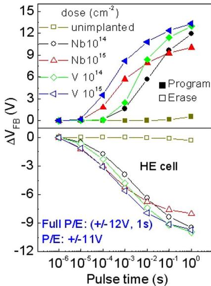
FIG. 3. (Color online) P/E characteristics of HE memory cells containing V and Nb ions of  $10^{14}$  and  $10^{15}$   $\text{cm}^{-2}$  fluences.
