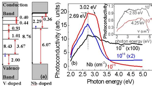
FIG. 1. (Color online) (a) Schematic diagram showing the calculated impurity energy levels for V and Nb doped  $\text{Al}_2\text{O}_3$ . (b) Photoconductivity spectra of HE memory cells containing V or Nb ions.
