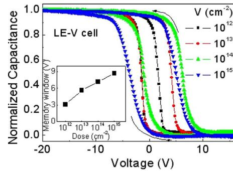
FIG. 2. (Color online)  $C$ - $V$  hysteresis loops of LE memory cells containing V ions of  $10^{12}$ – $10^{15}$  cm<sup>-2</sup> fluences. The inset shows memory window as a function of fluence.
