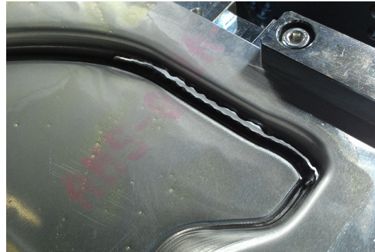
Figure 4.4: Tearing of the walls of the seat base when using single pass forming
