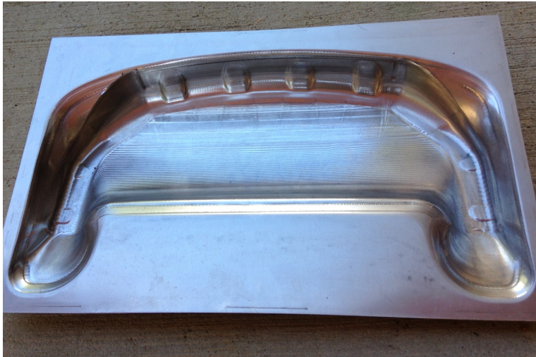
Figure 4.12: Photograph of the third attempt of the seat base component, successfully formed without cracks using bottom-up multi-pass SPIF
