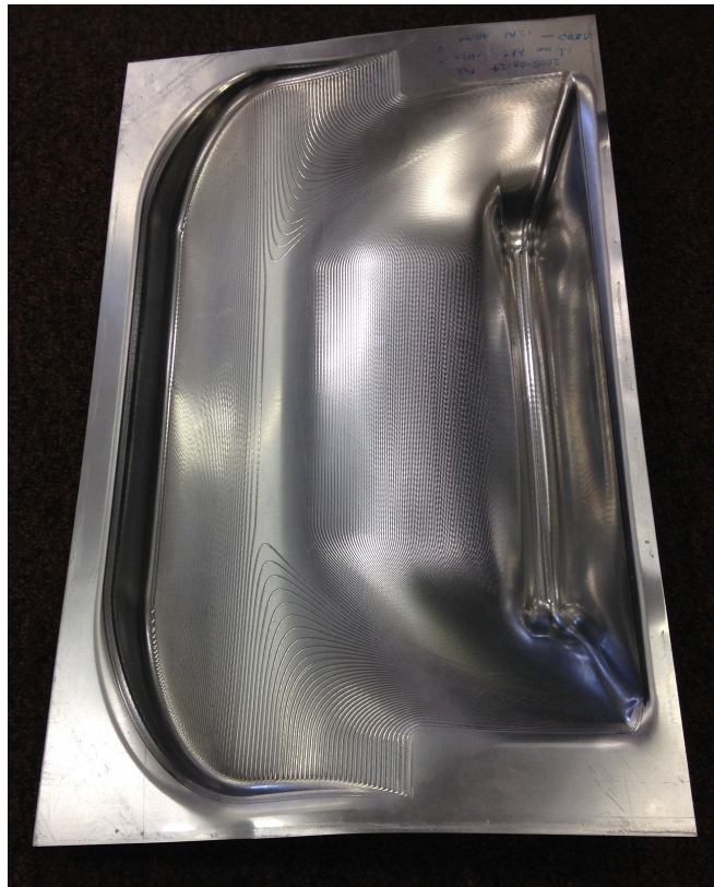
Figure 4.22: The cushion pan component, successfully formed with SPIF.
