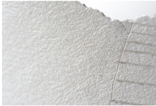
Figure 5.12: Close up of part near the point of fracture. The surface is regular and free of microcracks.
