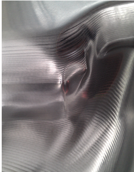
Figure 4.13: Detail of wrinkling resulting from the multi-pass forming of the first attempt for the seat base component.
