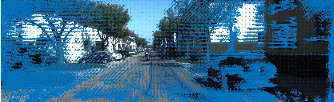
Figure 2.8: An example of optical flow computed using MATLAB 's Farneback optical flow function. The input images are taken from KITTI odometry dataset [Geiger et al., 2012], where the camera is moving forward. The blue arrows show the direction and magnitude of the pixels' motion between two consecutive frames. Note that the areas with no texture ( e.g. walls of building) has no optical flow due to the difficulty in computing optical flow within those regions.
