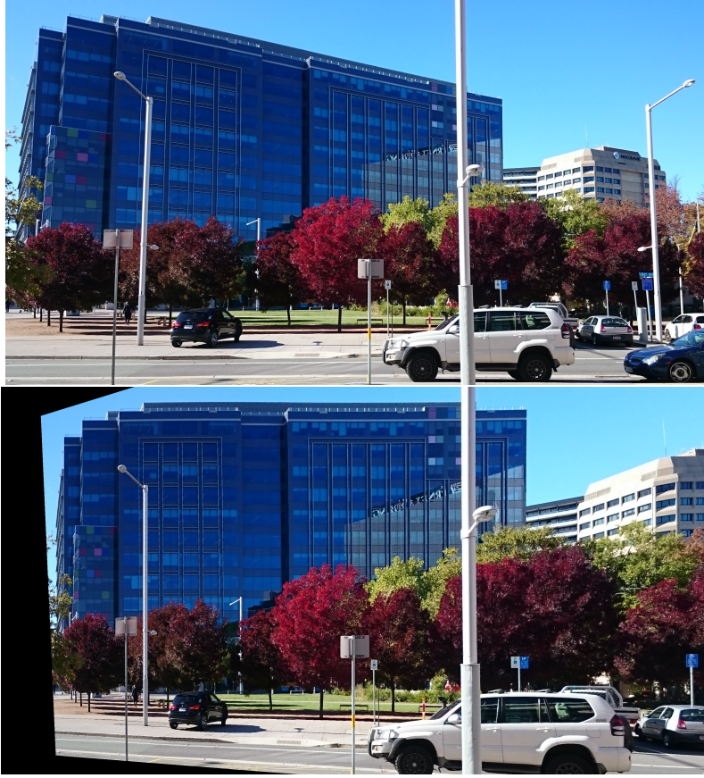
Figure 2.5: An example of removing projective distortion (of blue building) from a perspective image of a plane. From top to bottom: (a) original image; (b) homography transformed image. Notice that the windows of the blue building has orthogonal edges after the homography transformation, but other objects not on the same plane may look distorted. There are also black border on the left of the transformed image due to missing information (outside of original image boundary).
