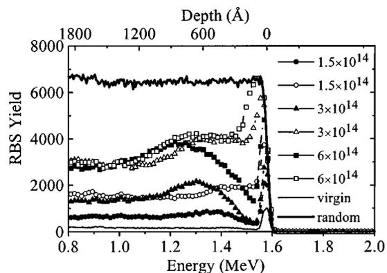
FIG. 1. RBS/C spectra showing the damage buildup for 0.5 MeV  $\text{Bi}_1$  (closed symbols) and 1 MeV  $\text{Bi}_2$  (open symbols) ion bombardment of GaN at 20 °C with a beam flux of  $\sim 1 \times 10^{11}$  Bi atoms/(cm<sup>2</sup> s). Implantation doses (in Bi atoms/cm<sup>2</sup>) are indicated in the figure.
