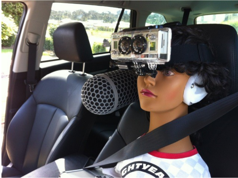
Figure 52: Binaural head with 3-D GoPro camera attached and Soundfield microphone in middle.
