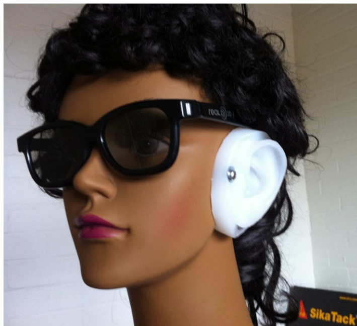
Figure 54: Custom made binaural head using mannequin head, silicon ears and condenser microphones inside ear canals.
