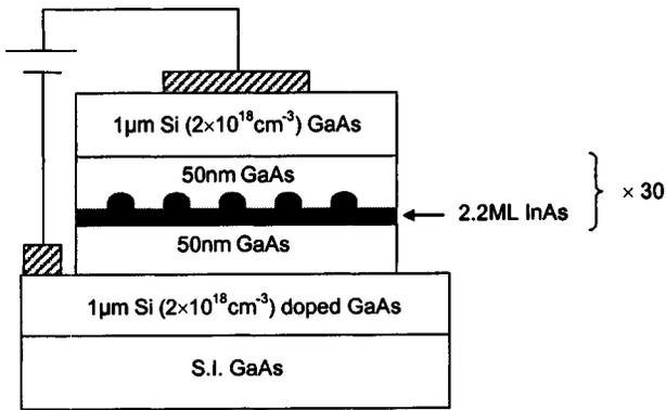
FIG. 1. Schematic of the quantum dot infrared photodetector.
