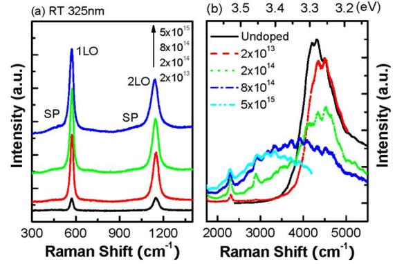
FIG. 3. (Color online) Resonance Raman spectra of As-implanted ZnO with different fluences in the ranges of (a)  $350\text{--}750 \text{ cm}^{-1}$  and (b)  $1800\text{--}5500 \text{ cm}^{-1}$ .
