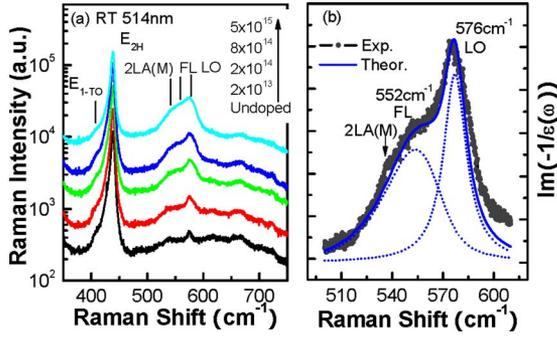
FIG. 2. (Color online) (a) Off-resonant Raman spectra of undoped and different fluence implanted ZnO. (b) The line shape fitting and experimental phonon peaks of As<sup>+</sup> implanted ZnO with a fluence of  $8 \times 10^{14} \text{ cm}^{-2}$ .
