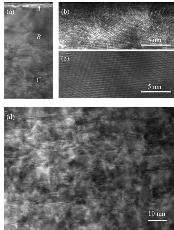
FIG. 1. (a) High-resolution bright-field XTEM image of 5 × 10<sup>15</sup> cm<sup>-2</sup> As<sup>+</sup> implanted ZnO single crystal, and (b)–(d) are the enlarged images of regions A–C denoted in image (a), respectively.
