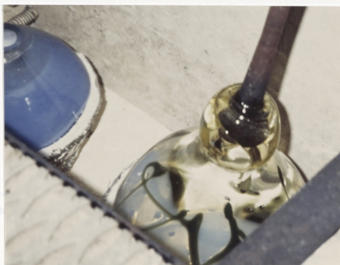
15) Cool piece gradually in annealing kiln.
