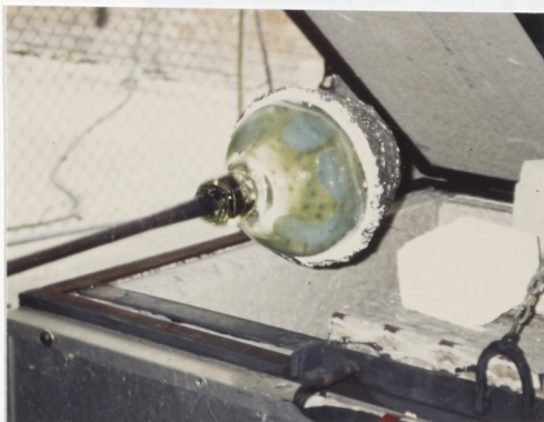
14) Put piece in annealing kiln, and knock off from pipe.
