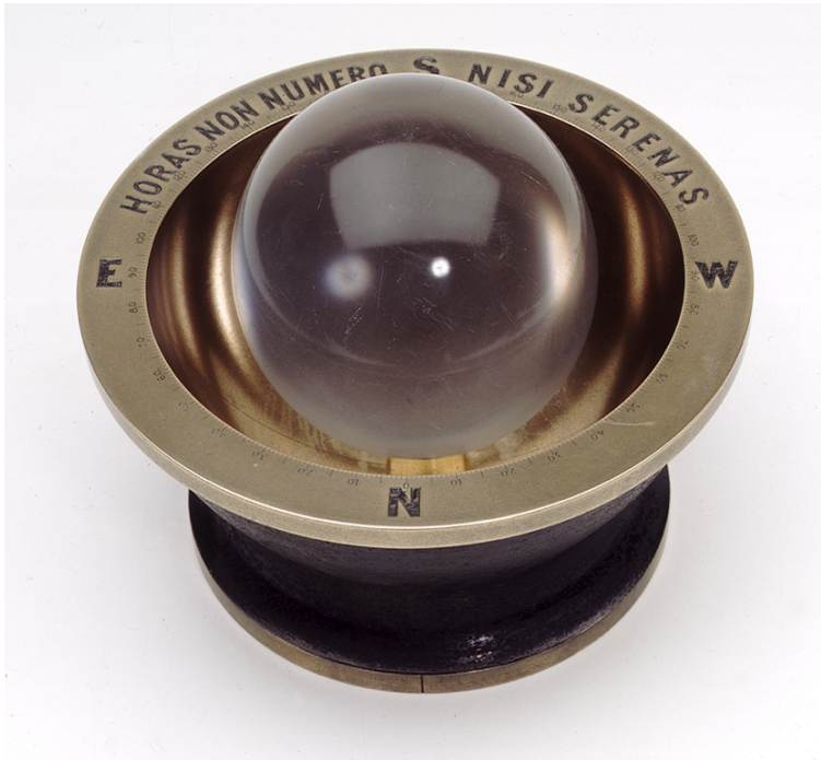
Figure 6.4.5 Sunshine recorder made by Mr. J. F. Campbell. 225
