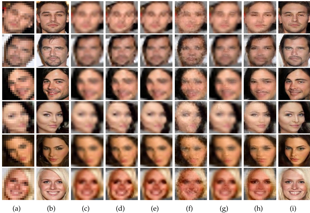
Figure 4.3: Comparison with the state-of-the-arts methods. (a) LR inputs. (b) Original HR images. (c) Bicubic interpolation. (d) The method of Yang et al. [2010]. (e) The method of Dong et al. [2016a] (SRCNN). (f) The method of Liu et al. [2007]. (g) The method of Yang et al. [2013]. (h) The method of Ma et al. [2010]. (i) Our method.
