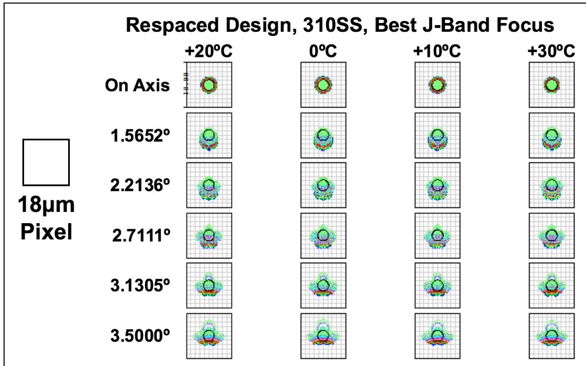
Figure 5: Spot diagrams across the field for the optical prescription, shown relative to the detector pixel size and as a function of temperature assuming detector refocus. The Airy circle for this system is represented by a black circle.
