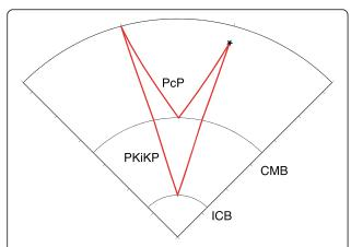
**Fig. 1** Ray paths of PcP and PKiKP seismic phases. A cross section of Earth with ray paths of PcP and PKiKP seismic phases originating at the source (*star*) and recorded by a station at the Earth's surface
