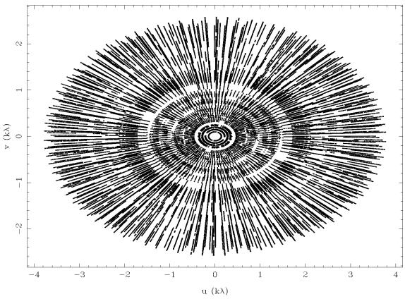
Fig. 1.— ATCA observing coverage in the uv-plane for a typical pointing in the 406-pointing mosaic. The central hole in the uv-coverage is filled by combining the ATCA observations with data from the Parkes 64 m telescope.
