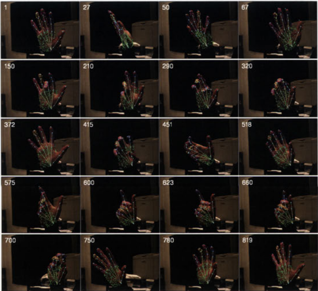
Figure 6.45: Selected frames from the collated sequence for tracking with the RVAR (relative) prediction model. 10000 iterations are used for each frame.
