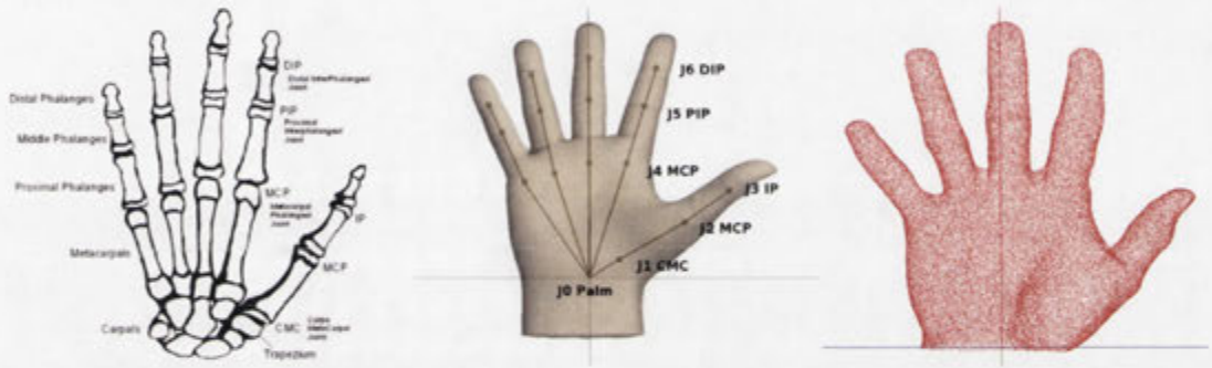
Figure 3.3: Left: Skeletal structure of the hand. (Image taken from McDonald et al. [52]) Middle: The hand model used for hand tracking. Right: The deformable mesh of the hand model.
