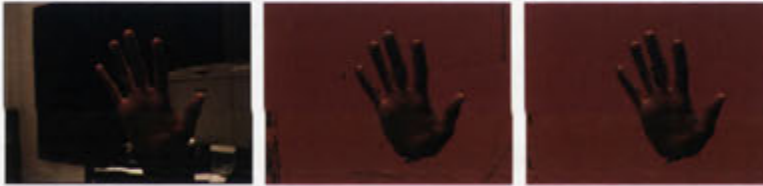
Figure 5.5: Left: Original image. Middle: Skin detection via a trained histogram model. Right: Noise removal and gap filling via dilation and erosion methods.
