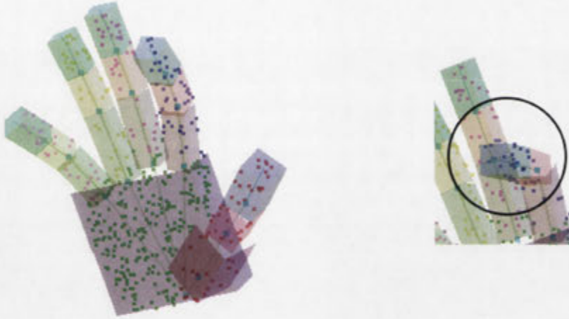
Figure 5.2: Left: Bounding volume model for the self-occlusion test. Right: Sample points on the middle finger (in red) occluded by the index finger (in blue) are discarded.
