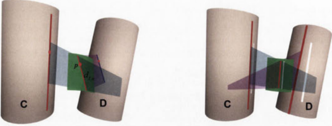
Figure 4.5: Left: The green surface is a patch of the hand segment that has been perturbed from \mathbf{x}^* . An active point p lies on a trajectory d_{1,\eta} (marked in red). The projection of d_{1,\eta} onto cylinder C lies on a line with a constant YUV value. The projection of d_{1,\eta} on cylinder D however will almost always lie on a curve (marked in blue) with a non constant YUV value. Right: A perturbation where both projections of d_{1,\eta} have the same YUV value. One can always choose active points from a neighbouring trajectory d' (marked in white) to increase C_{\mathbf{x}^*} , due to the foreshortening effect of cylinder D observed from camera 2.
