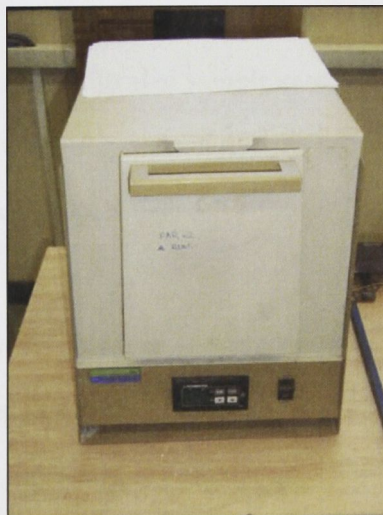
Figure 4.10: Small furnace used to cure infiltrated samples, Materials Laboratory, Department of Engineering
