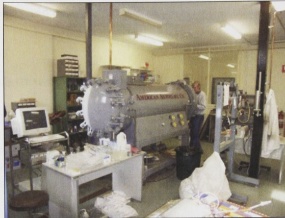
Figure 4.11: Autoclave used to cure infiltrated samples, Materials Laboratory, Department of Engineering
