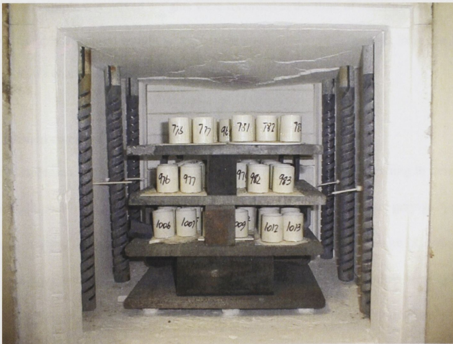
Figure 4.6: Group A, pre-firing in ANSTO Laser dilatometer furnace, 1300°C, showing silicon carbide shelving and high alumina sheeting
