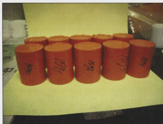
Figure 4.9: Cylinders of hardened polymer/mineral composite, each containing an infiltrated sintered sample
