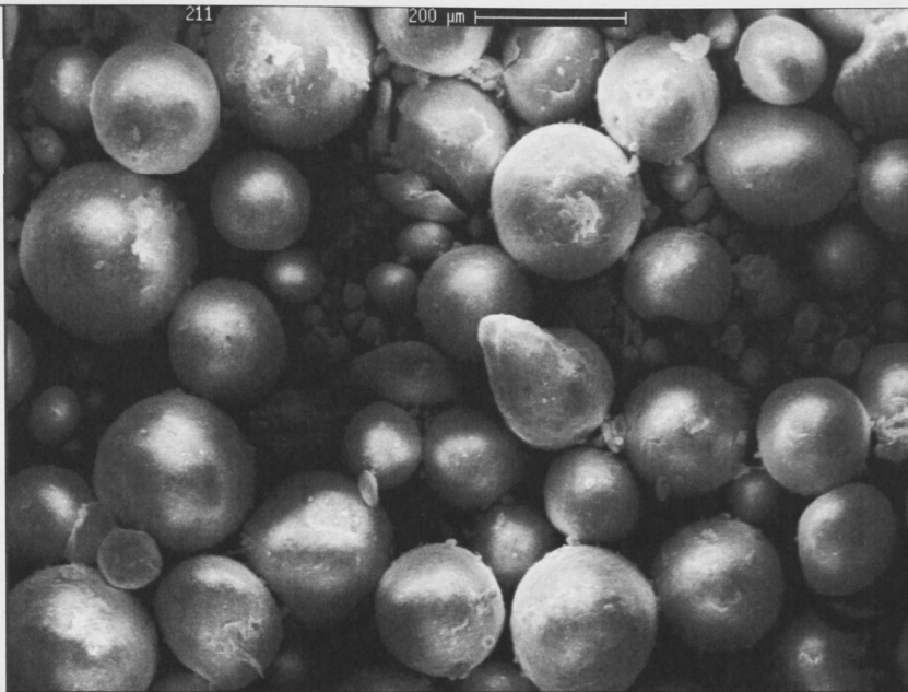
Figure 4.3: Electronmicrograph of silica fume particles, x100
