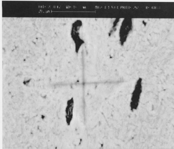
Figure 4.7: High-magnification BSE image of the indentation pattern (0.49N), 1500x
