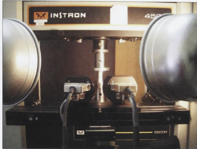
Figure 5.1 Experimental set up for compression test
