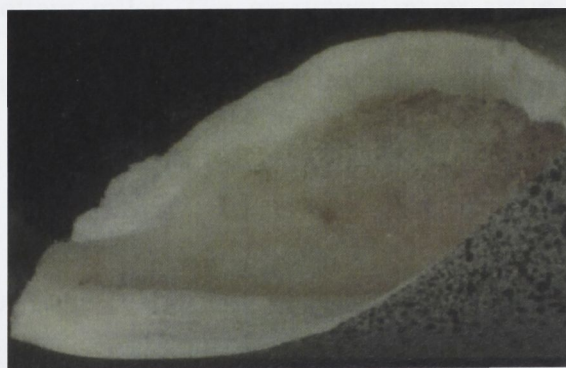
Figure 6.6: Typical damage in sample loaded at 1.3 mm/min
