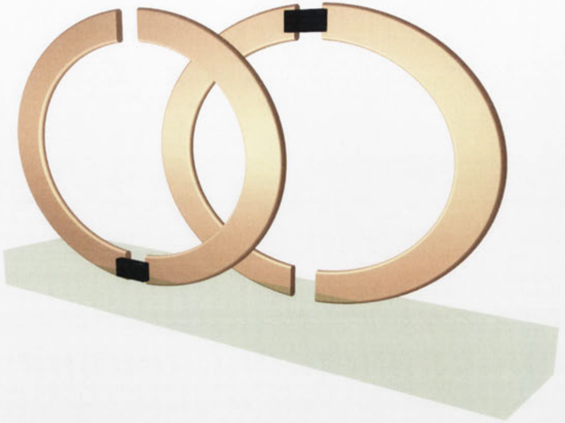
Figure 3.5: Schematic of the SRRs inside the plexiglass stand.
