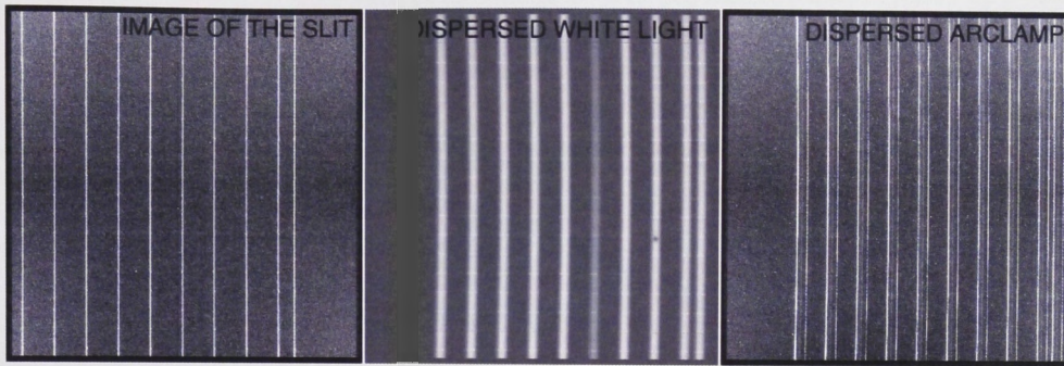
Figure 5.4 Calibration frames. Each vertical line is comprised of 19 nearly-adjacent slitlets. Using this 10 \times 19 grid of slitlets, we imaged the grid (left), added a grism to the light path to disperse the white light (center) and illuminated the 190 slitlets with a HeAr lamp and dispersed the light (right). In combination, these three frames allow us to map the anamorphic distortion, measure the bandpass shift as a function of CCD position and calculate the local dispersion.
