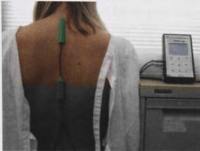
Figure 1: Flexible electrogoniometer attached to the upper thoracic spine with datalog on the right
