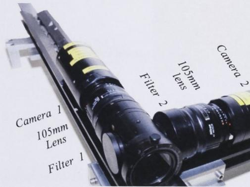
Figure 3.5: Collection optics for the helium line ratio diagnostic.
