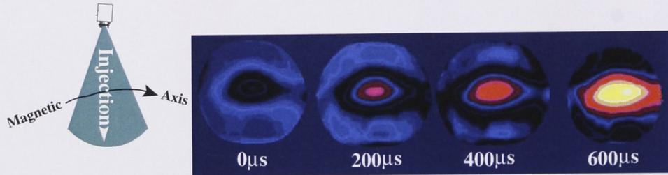
Figure 5.17: Raw light images, corrected for vignetting, taken through the optical view port as the injection was initiated.
