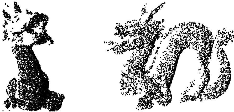
Figure 4.4: Two partially-overlapping point-sets from the DRAGON-STAND dataset of the Stanford Computer Graphics Laboratory. The point-sets were captured from two different locations and do not overlap completely, making them challenging to register accurately.
