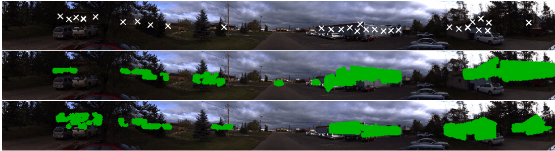
(b) Panoramic photograph and extracted 2D features (top), building points projected onto the image using the RANSAC camera pose (middle) and building points projected using the GOPAC camera pose (bottom).
