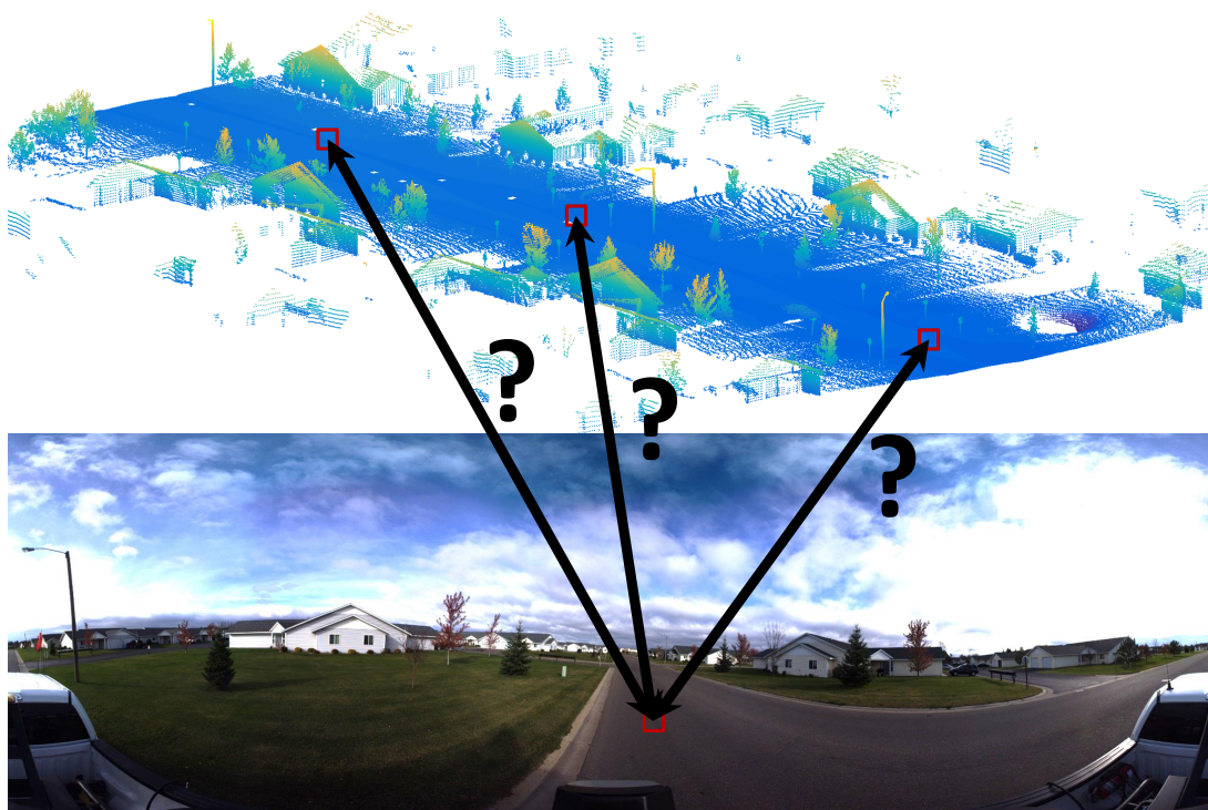
Figure 6.2: The cross-modality correspondence problem. 2D–3D correspondences are difficult to obtain, particularly across modalities. In the situation illustrated here, the point-set was captured by a laser scanner and has no visual information associated with it, making the correspondence problem challenging.
