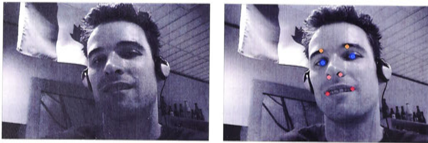
Figure 2.22: Face registration. (a) An image containing a face. (b) Presence of face verified and facial features detected. This example is from our system described in Chapter 5
