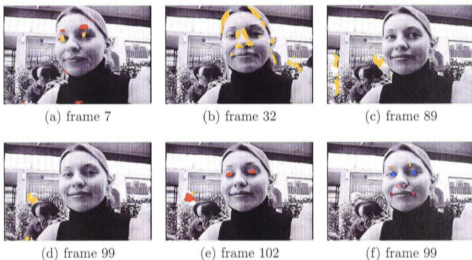
Figure 5.22: Snapshots of a sequence. Regions of motion are indicated in yellow and blink-like motion is indicated in orange.
