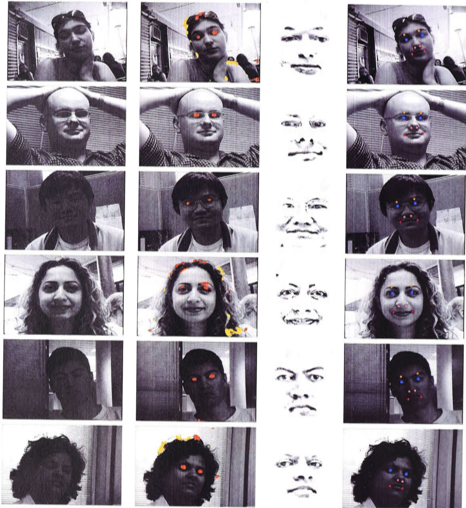
Figure 5.23: Results of the system on a range of subjects. The first column shows the raw image where eye motion is detected, the second column show the motion regions, the third column shows the enhanced facial region extracted, and the fourth column shows the features detected.
