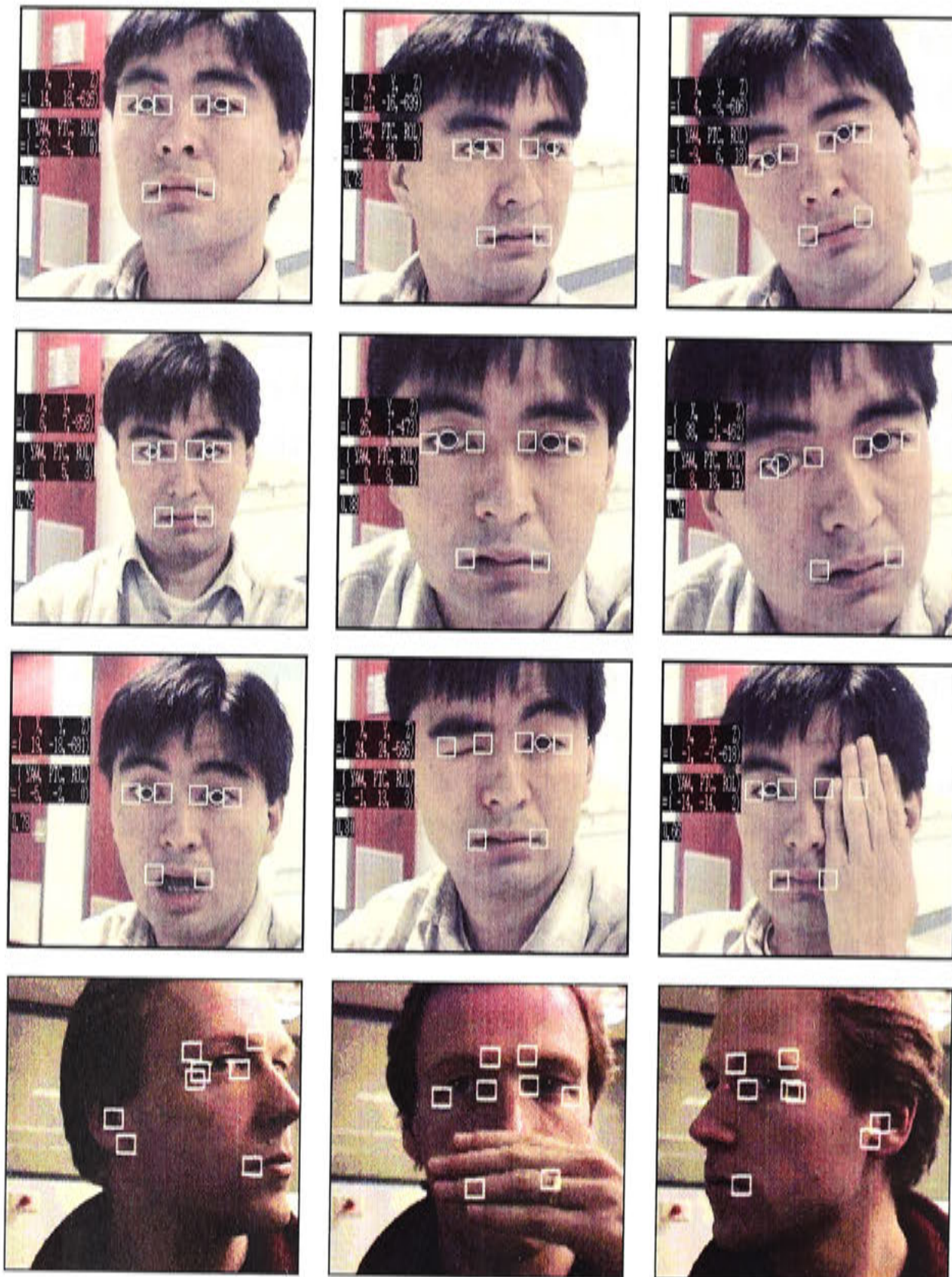
Figure 2.27: Example of Matsumoto and Zelinsky's system tracking the 3D pose of the head.
