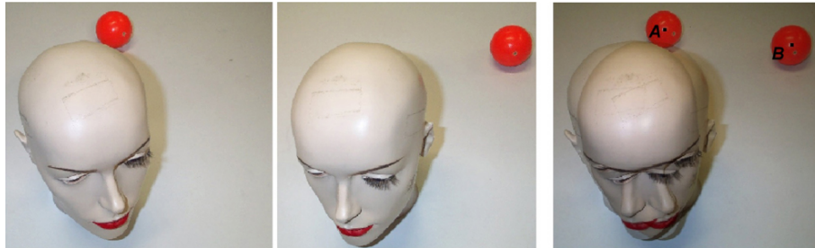
Figure 6.2: An example of binocular disparity. The insets show (from left) the left and right camera views and an overlay of left and right views. Gaze is fixated upon the mannequin’s forehead. Vector A-B represents disparity for the ball. The images have not undergone parallel epipolar rectification, so there is a vertical component to the disparity vector. A wide baseline introduces parallax disparity at the mannequin’s face.
