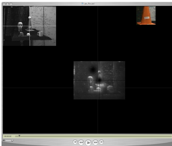
Figure 8.25: Online dynamically updated fixation map demonstration ( snapshot - see Appendix C for full video ). The insets show the rectified camera image (left) and selected target extraction (right).
