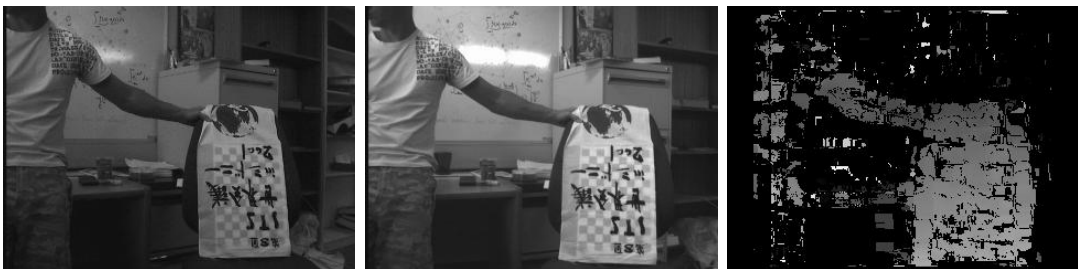
Figure 8.6: Disparity cue. Left and right input images, and resulting disparity map (respectively).
