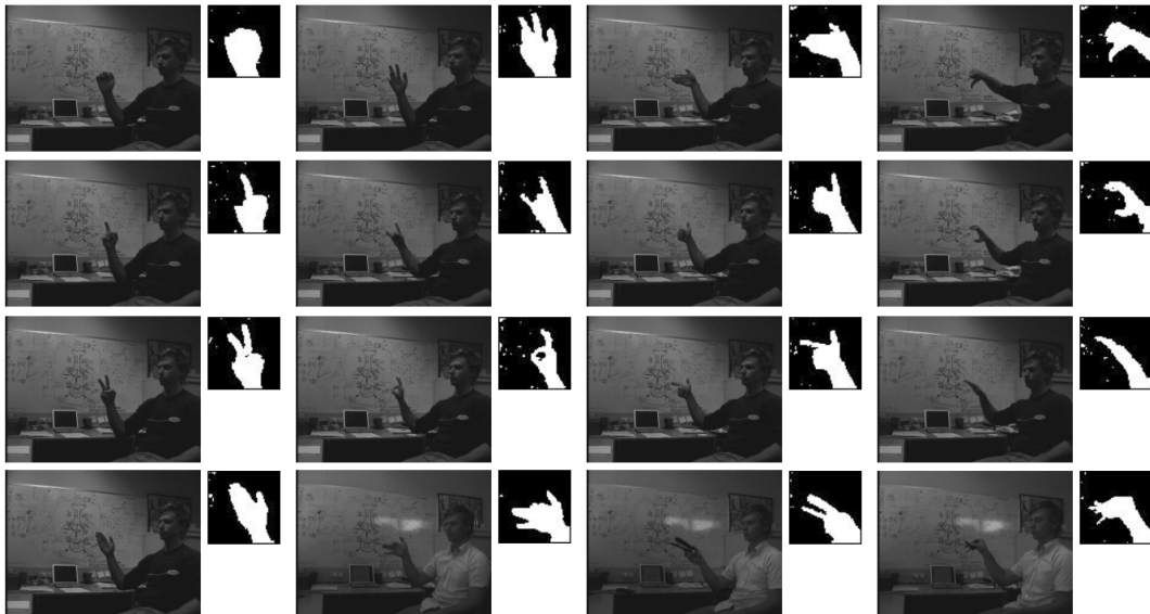
Figure 7.11: Segmentation of objects with intricate borders. The last two frames show composite objects - a hand grasping a stapler, and a hand grasping a bunch of keys.
