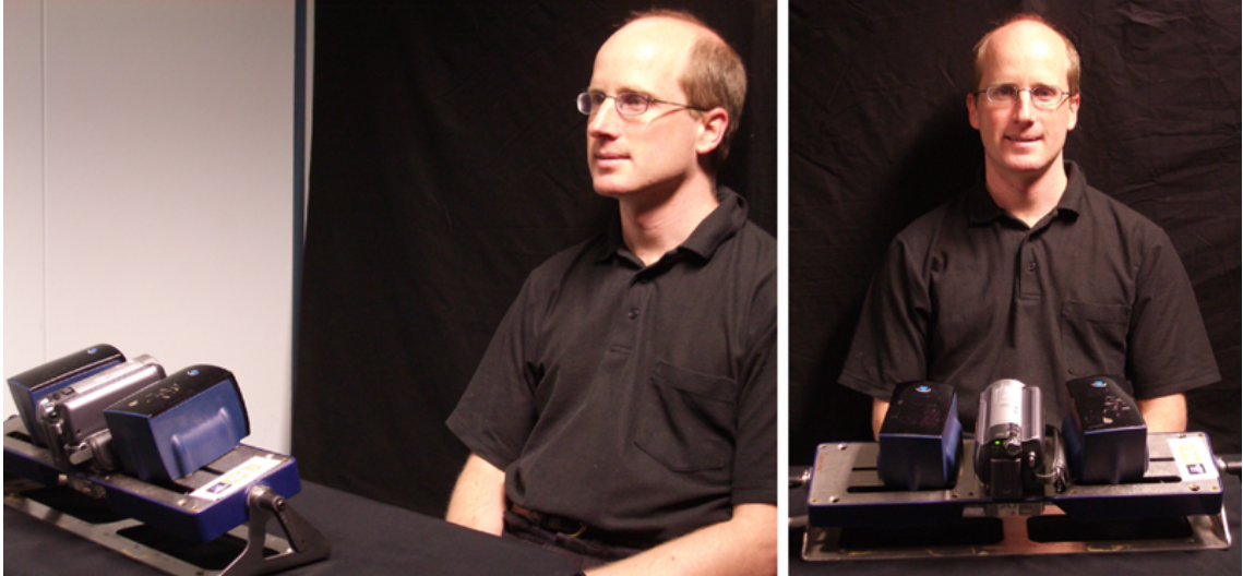
Figure 9.5: Non-intrusive acquisition of participant's 3D gaze path using FaceLAB. An extra video camera is used to record the participant, placed between FaceLAB cameras.
