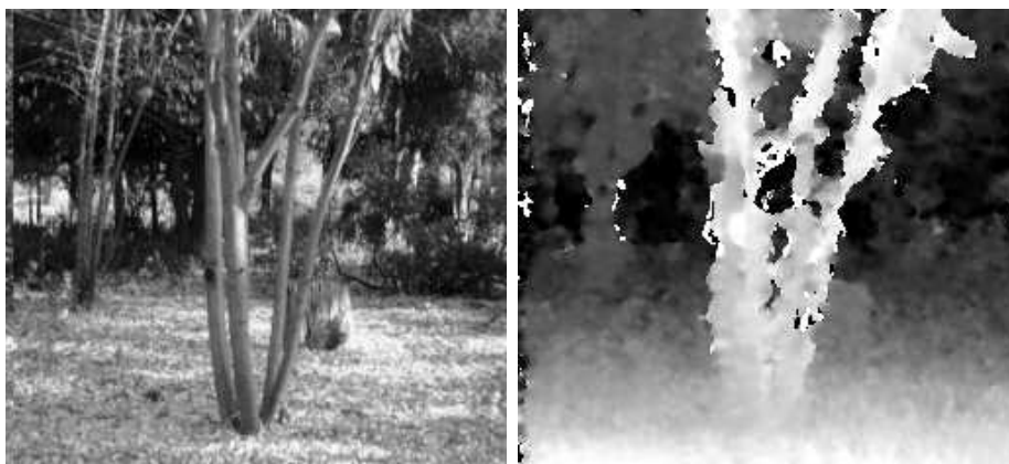
Figure 6.4: Example disparity map. One of the input camera views (left), and a dense disparity map output (right). Distant scene regions are represented by darker intensities.
