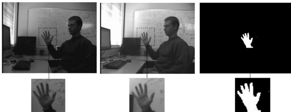
Figure 7.1: Foveal object segmentation and coordinated fixation. The left and right input (respectively), and the output from the Markov random field zero disparity filter (MRF ZDF).
