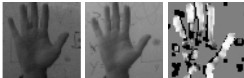
Figure 7.4: Correlation-based ZDF output. NCC of 3 \cdot 3 pixel regions at same coordinates in left and right images. Higher correlation values are shown more white.
