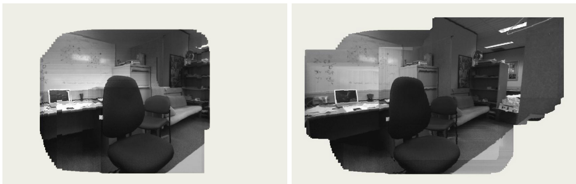
Figure 5.1: Online output of the active rectification process. Mosaics of rectified frames from right CeDAR camera at time 10sec, (left) time 20sec (right).
