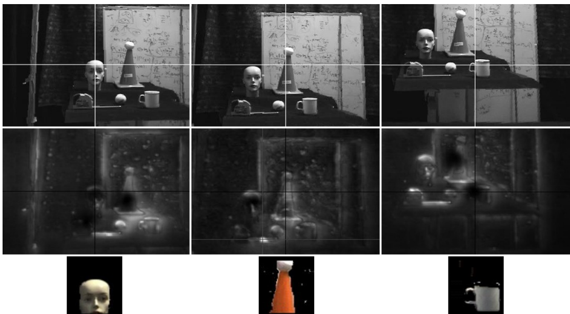
Figure 8.24: Sample system behavior. Each column shows camera image, fixation map and MRF ZDF segmentation. From left: 1 attention shifts to head from inhibited base of cone, forehead is segmented from background in fovea; 2 attention returns from inhibited head to top of cone, cone is segmented; 3 attention shifts from inhibited cone to mug, mug is segmented.
