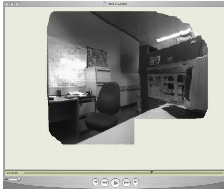
Figure 5.11: Online image rectification and mosaicing, left camera. In this demonstration, the camera was moved by hand while the images were automatically rectified ( snapshot - see Appendix C for full video ).
