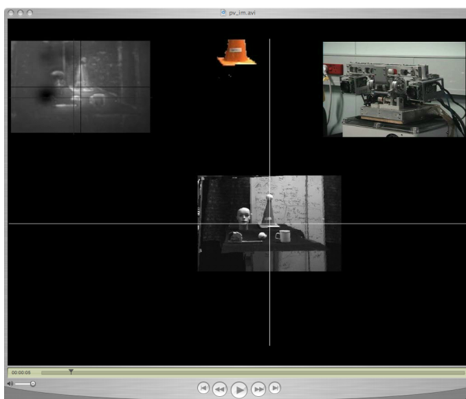
Figure 8.26: Online system demonstration showing image mosaicing ( snapshot - see Appendix C for full video ). The insets show the fixation map (left); target extraction (centre); and the active head (right).
