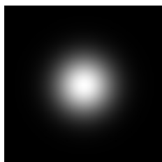
Figure 8.14: Gaussian IOR increment pattern. This kernel is applied at the coordinates of the centre of each view frame in the IOR accumulation mosaic (centre, Figure 8.20).
