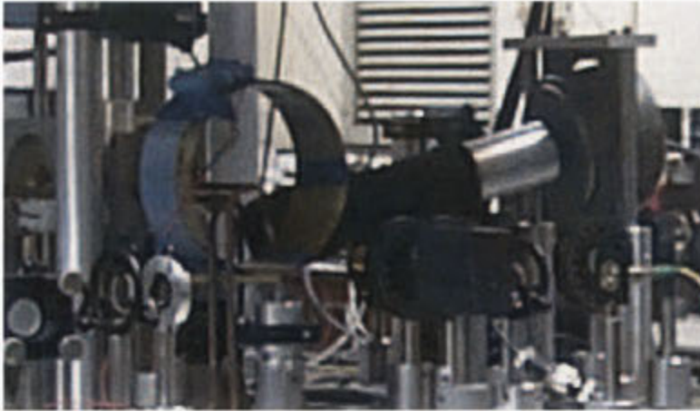
3.6: The imaging optics and CCD camera. The CCD camera can be seen in the background. Much of the imaging optics is ensconced within the general laser cooling optics.
