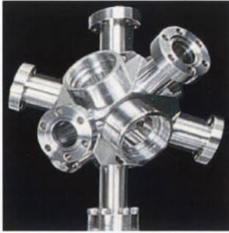
4.2: Photo of the ANU-BEC-I collection chamber. The chamber is a truncated cube: the six large faces hold indium-sealed optical quality windows for the MOT beams; the eight tubes provide 1 1/3" conflat connections used for: connecting the chamber to the rest of the vacuum system; an electrical feedthrough driving the Rb dispensers; and windows for the push beam and general observation.
