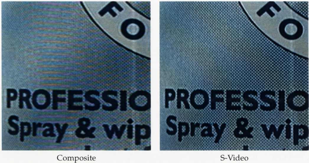
Figure 4.3: Comparison of S-Video and Composite Video
