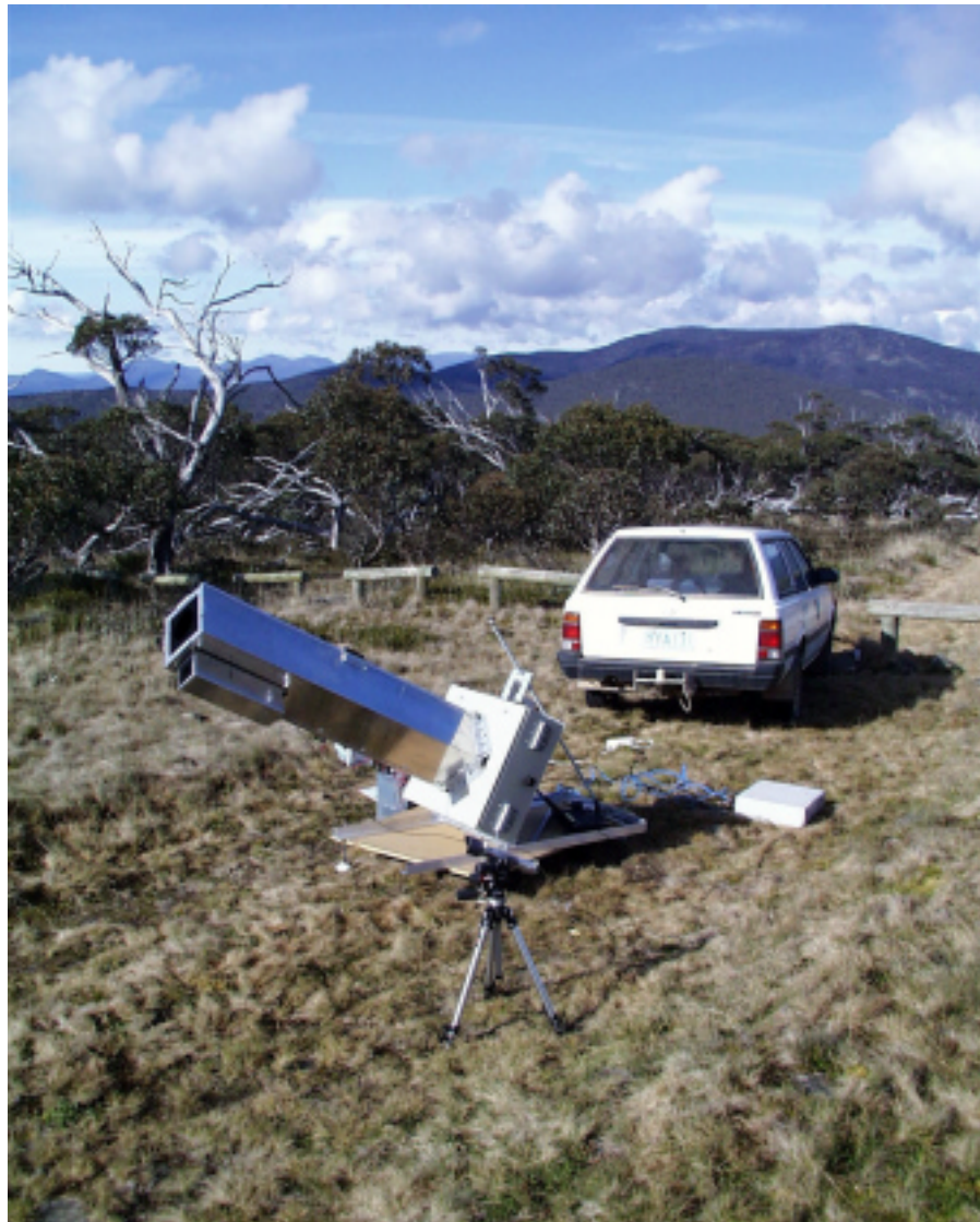
Figure 2-1: Calibration of solar cells under natural sunlight at Mt Ginini (1762 m), ACT, Australia. This picture was taken during experimental verification of the method, at a high altitude site.
