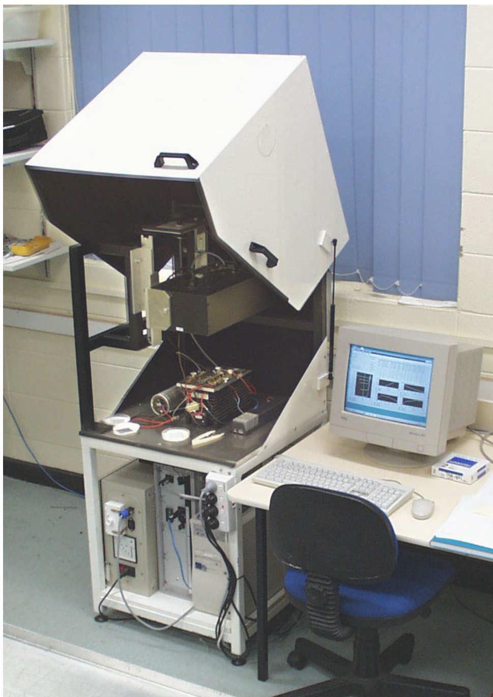
Figure 3-1: The constant voltage flash testing system.
