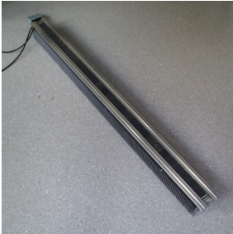
Figure 1-2: An air-cooled PV/Trough receiver (1.7m long). 31 cells produce approximately 20V/12A at 20X.
