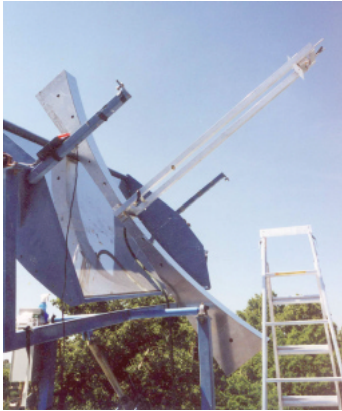
Figure 3-16: The segmented parabolic trough constructed for measurement of cells under concentrated natural sunlight. It is piggybacked on the tracker for a normal, full-length parabolic trough mirror.
